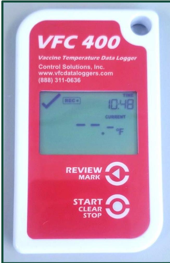
If this error displays on the data logger screen after starting back up, it is because the device was NOT plugged into the unit before restarting it. You will have to stop the data logger and dock it again to reconfigure.
